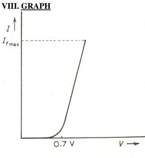
Forward characteristics of a silicon diode
