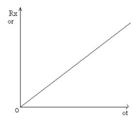
Transmitter Rotor Position Vs Receiver Rotor Position
