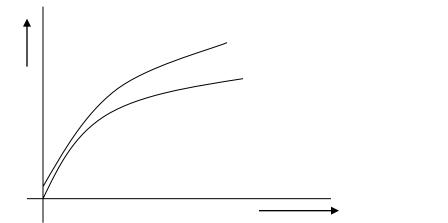
**Internal Characteristics**: It is the characteristic drawn between  $E_g$  and  $I_a$  ( $I_a=I_L=I_{se}$ ).
