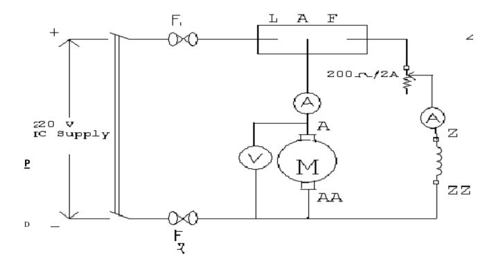
2. Start the motor slowly using starter keeping the field and armature rheostats in minimum and maximum position respectively.
